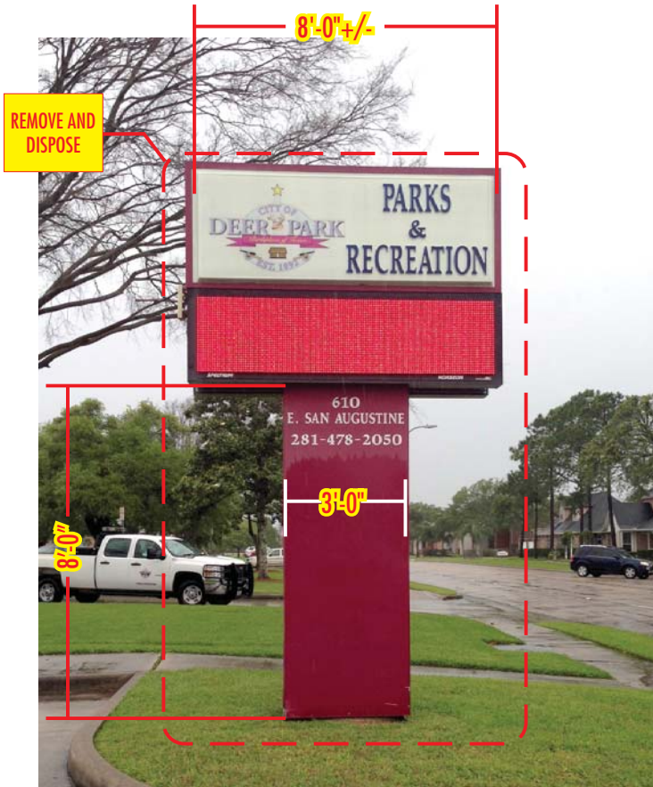
SIGN ELEVATION: SIDE A EXISTING CONDITIONS SCALE: 3/8" = 1'-0"
