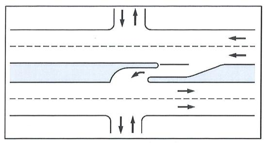
Figure 2: Left-Turn Ingress from One Direction
