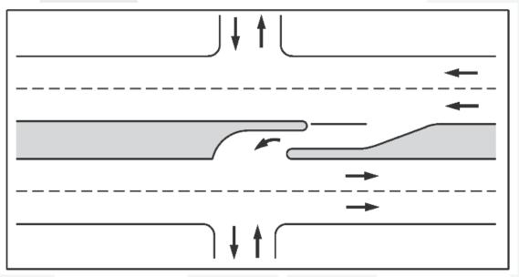
**Figure 2: Left-Turn Ingress from One Direction**
