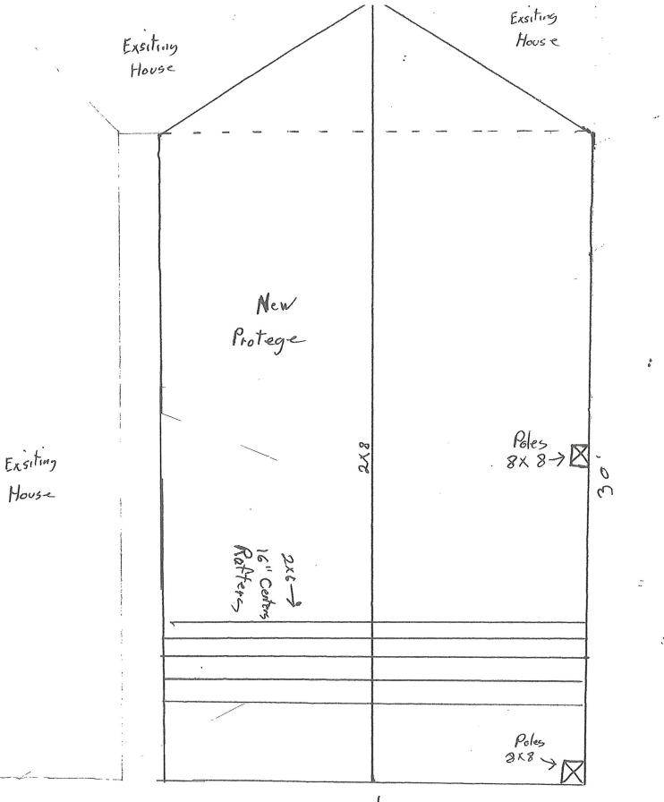
Dobbul 2×12 2112 2X8 Handy 216 Raffle. 2×6 Joist 12 Plywood . Comp Shingle Plywood / Sawfit 10 Concrte.
