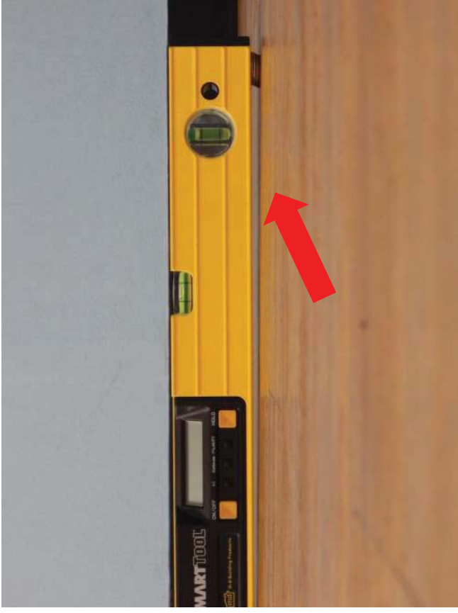
#43 Level on floor showing sloping down toward the North East corner at Approximately 1/8" per foot
