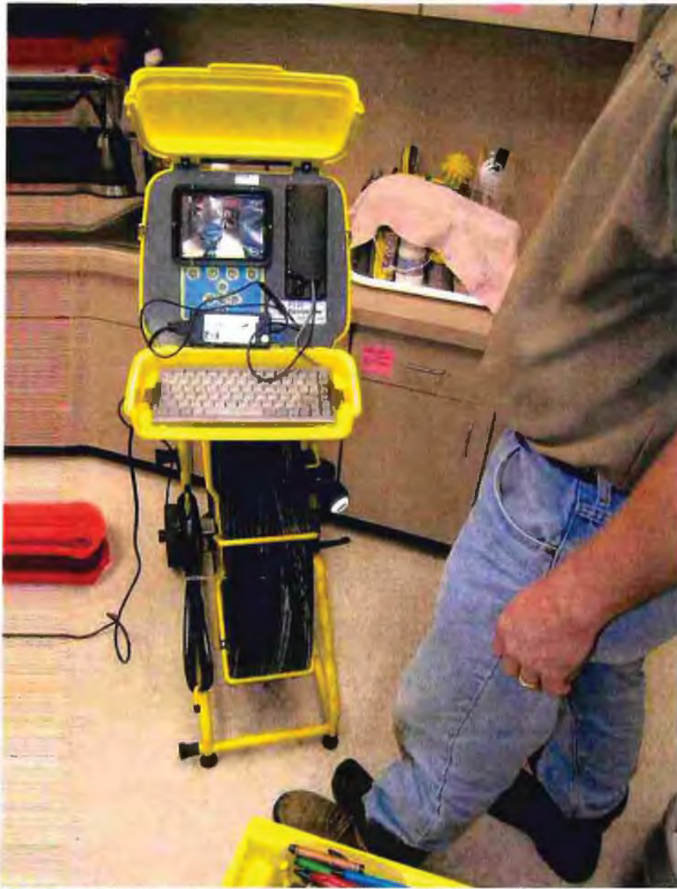
Video inspection of underground sanitary plumbing in addition.
