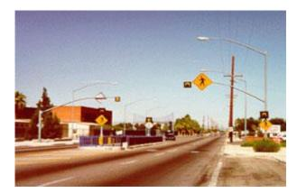
Figure 40. Fences or railings in the median direct pedestrians to the right and may reduce pedestrian crashes on the second half of the street.
