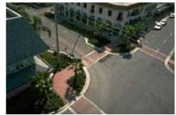
Figure 35. Curb extensions at intersections reduce crossing distance for pedestrians.
